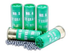
SHOT SHELL: No. 1, 3, 4, 5 or 6 GAUGE: 12 HEAD BRASS: 16 mm CASE: 70 mm LEAD: 35 gram WAD: PLASTIC SHOT SIZE: 1, 3, 4, 5, 6 CRIMP: \* BOX: 25/250 VELOCITY AT MUZZLE: 360 m/s SHOT SHELL: No. 1, 3, 4, 5 or 6 GAUGE: 12 HEAD BRASS: 16 mm CASE: 70 mm LEAD: 32 gram WAD: PLASTIC SHOT SIZE: 1, 3, 4, 5, 6 CRIMP: \* BOX: 25/250 VELOCITY AT MUZZLE: 365 m/s
